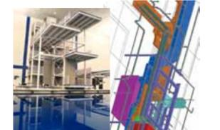
Building Information Modeling was used for shoring of the concrete decks for the dive tower platforms and to provide a layout for support beams. The shoring was built to support the concrete formwork for the platforms.
